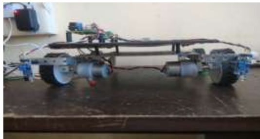
Figure 4.1: Model on Detecting Crack in Railway Track
