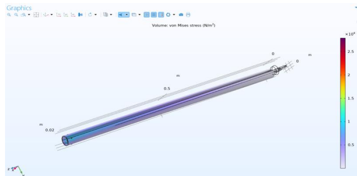
Stress Acting on the Arm of Multirotor UAV
