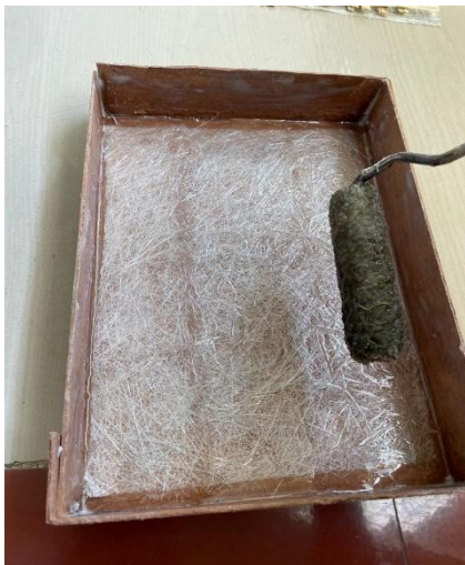
Rolling is done to Remove Air Trapped Inside & Spreading Epoxy
