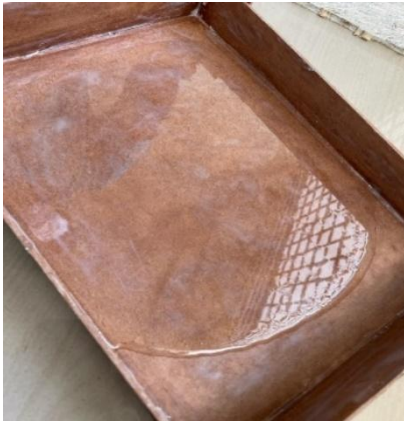
First the Epoxy Mixture is Poured which is Mixed in the Ratio of 1:3
