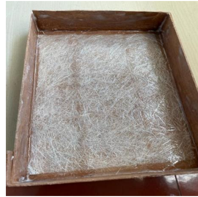
Glass Fiber Sheet Placed Over Epoxy
