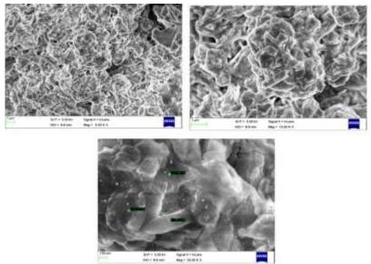
Figure 4 SEM Images of Ni<sub>0.2</sub>Co<sub>X</sub>Fe<sub>2-X</sub>O<sub>4</sub> (X=0.1, 0.3)
