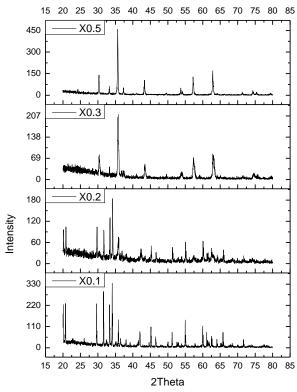
Figure 1 X-ray diffraction pattern of Ni0.2Co<sub>X</sub>Fe<sub>2-X</sub>O<sub>4</sub>
