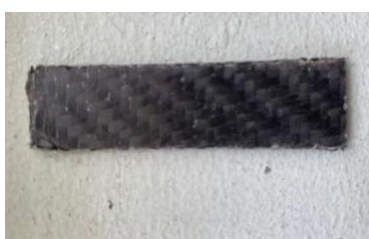
Figure 4: Specimen B Length: 55 mm Width: 10mm Thickness: 5mm
