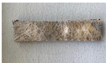
Figure 3: Specimen A Length:55 mm Width:10 mm Thickness:3mm
