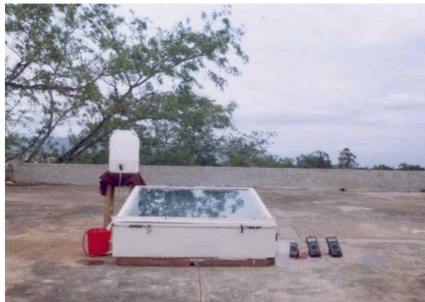
Figure 1 Photograph of the Perched Cum Off-Centered Wick Solar Still
