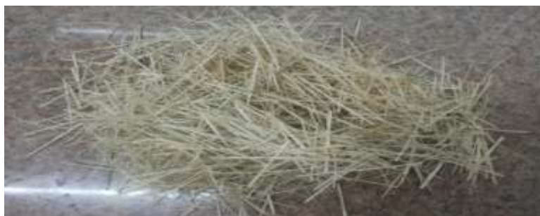
Figure 4: Dia 1.156 mm fiber of aspect ratio (l/d)-40
