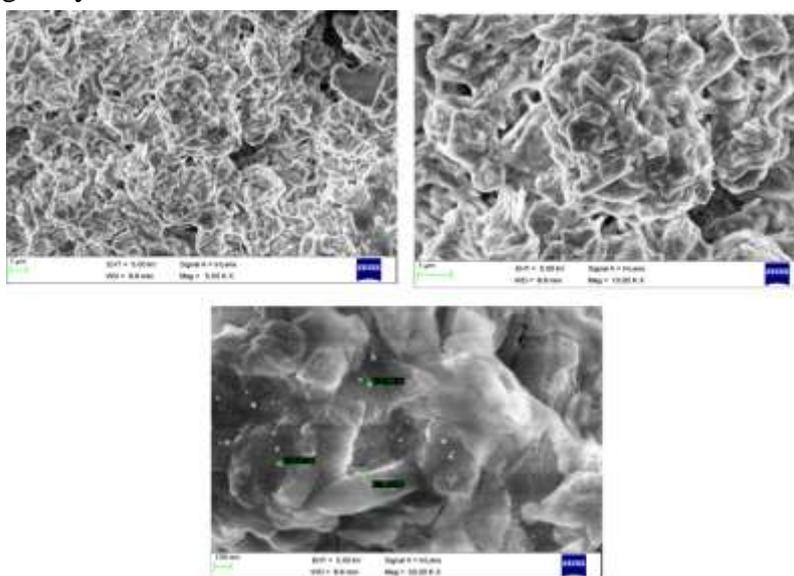
Figure 4 SEM Images of  $\text{Ni}_{0.2}\text{Co}_x\text{Fe}_{2-x}\text{O}_4$  ( $X=0.1, 0.3$ )
