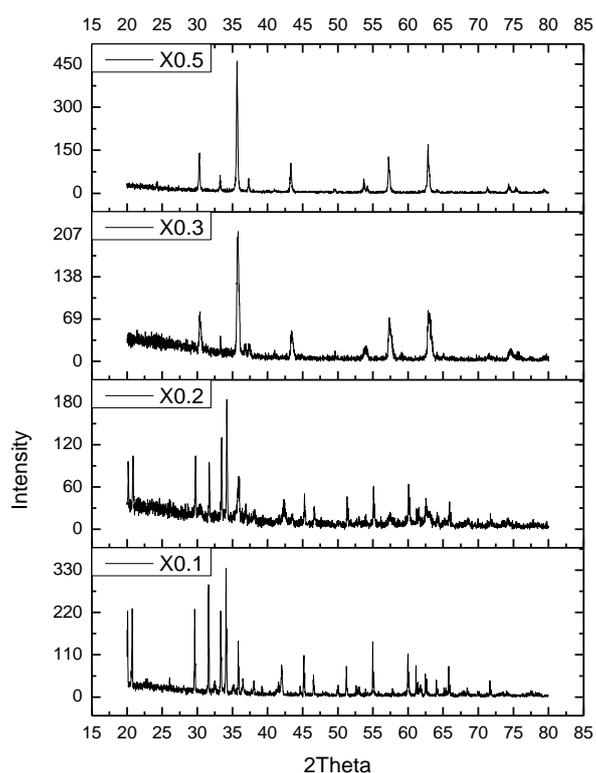
**Figure 1 X-ray diffraction pattern of Ni<sub>0.2</sub>Co<sub>x</sub>Fe<sub>2-x</sub>O<sub>4</sub>**
