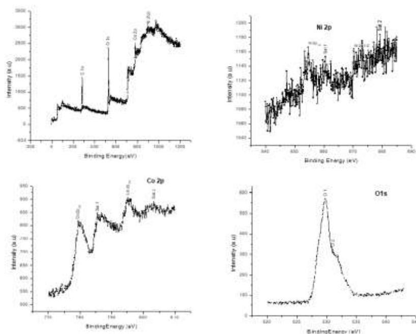
**Figure 2 XPS Spectrum of [a] Survey spectrum, [b] Ni 2p spectrum, [c] co 2p spectrum [d] O1s Spectrum for the NiCoO<sub>2</sub>**
