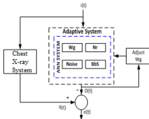
**Figure 2 Proposed Adaptive Filter Based Noise Cancellation System (AFNCS)**
