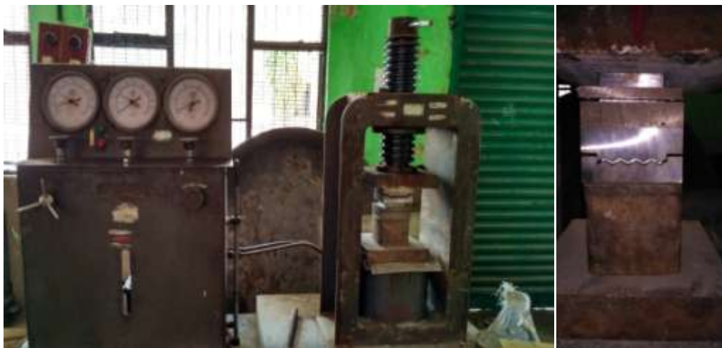
Figure 1: a) Hydraulic Press and (b) Specimen Sandwich between the Corrugated Die and Flat Die
